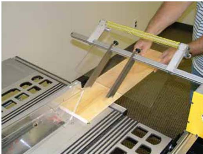
Feeding Stock Under Saw Guard
